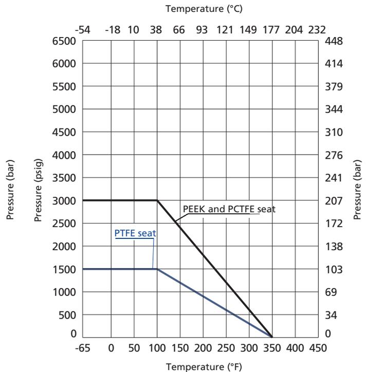
Note: The working pressure of valves is restricted by materials of the valve body and seat, as well as end connections. When choosing a valve for your applications, please refer to the above Temperature vs. Pressure Curves and the pressure rating in the dimension table. The minimum value shall be the pressure rating of the valve.
