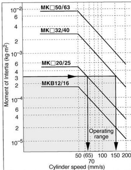
When arm's inertia is  $3 \times 10^{-4} \text{kg}\cdot\text{m}^2$ , cylinder speed should be less than
