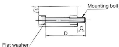
Note) Be sure to use a flat washer to mount ø12 and ø16 cylinders via through holes.
