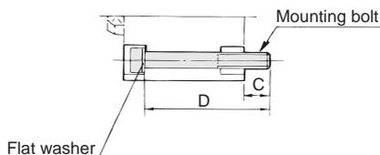
Note) Be sure to use a flat washer to mount cylinders via through holes.
