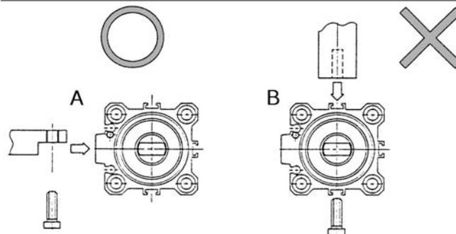
\*When installing the arm for the parallel section at the rod end, the strength of the piston rod might be insufficient depending on the direction in which the arm is installed. Therefore, make sure to install the arm in the direction indicated in diagram A.
