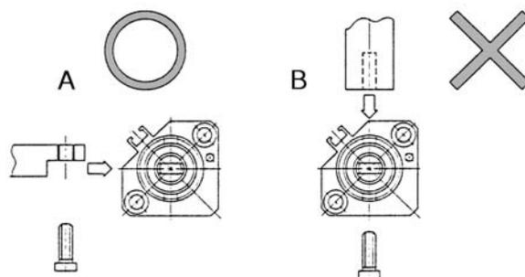
\*When installing the arm for the parallel section at the rod end, the strength of the piston rod may be insufficient depending on the direction in which the arm is installed. Therefore, make sure to install the arm in the direction indicated in diagram A.
