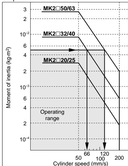
When arm's moment of inertia is  $5 \times 10^{-3} \text{kg/m}^2$ , cylinder speed should be less than
