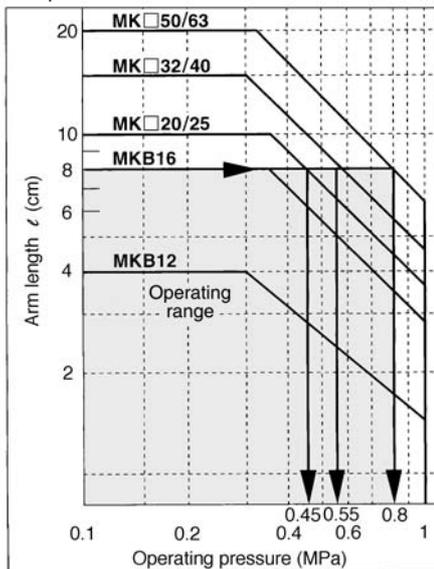
When arm length is 8cm, pressure should be less than
