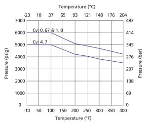
The temperature rating of CH Series check valve is restricted by the connection types. For details please refer to B-134.
